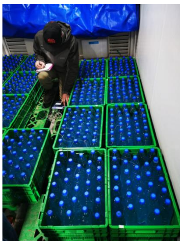
Figure 1. Example stacking of crates of dummy load water bottles in a WICR. Note that a 100mm air gap should be allowed between any crate and a nearby wall.
