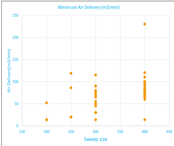
Figure 11: Range of air delivery based on sweep size for table & wall mounted fans
