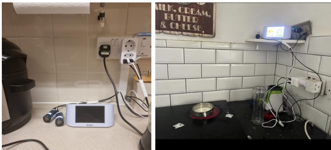
Figure 2.3 typical placements of active NO 2 and CO sensors and the PM 2.5 /CO 2 sensor. Left photo: the passive NO 2 tube can be seen at the top fixed to the tiles.
