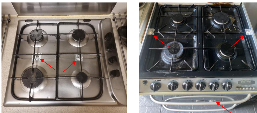
Figure 2.2 Left: ideal placement of iButtons on gas hob. Right: due to the construction of the gas hob the two iButtons could not be placed between the burners and had to be placed on the sides. Note: on the oven door a third iButton was placed.
