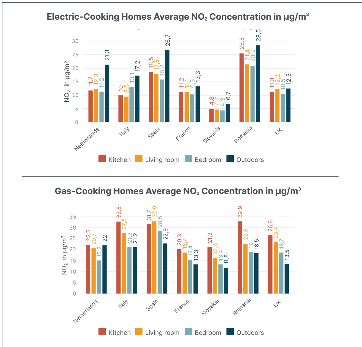
FIGURE 6. AVERAGE NO 2 CONCENTRATIONS PER COUNTRY AND PER COOKING METHOD IN DIFFERENT ROOMS
