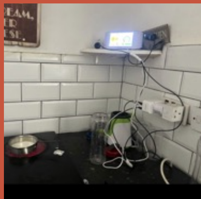
FIGURE 4. TYPICAL PLACEMENTS OF NO 2 AND CO SENSORS, THE PM 2.5 /CO 2 SENSOR, AND PASSIVE NO 2 SENSORS
