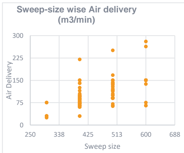
FIGURE 9: Range of air delivery based on sweep size for pedestal fans
