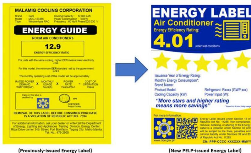
In June 2021, the Philippines adopted the PELP Implementing Guidelines, which include the new star-rating label (blue and yellow label, Figure 1) requirement for air conditioners, refrigerating appliances, lighting products, and TVs. Frequent revisions to the label criteria to keep up with market and technology trends will be essential to maintaining the value and integrity of the PELP program and shifting the Philippine market towards more efficient products.
