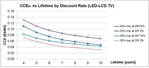
Figure 3. Sensitivity to lifetime and discount rates of cost per unit of conserved electricity ( $CCE_m$ ) for 1D backlight dimming
