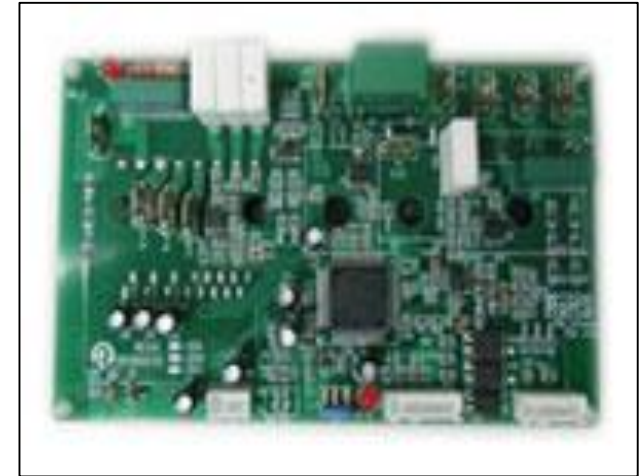
Compressor driver board
