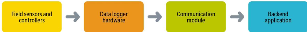
Figure 11: A basic block diagram of a remote monitoring system.
