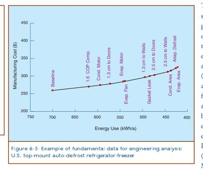
The seventh and final step in the analysis is to generate cost-efficiency curves. Figure 6-5 illustrates the results of an engineering/economic analysis for an 18.2-ft<sup>3</sup> (515-liter), top-mount, auto-defrost refrigeratorfreezer. In large part, this analysis was used as the basis for the consensus efficiency standards established by U.S. DOE in July 2001 (U. S. DOE 1995). Manufacturing cost is
