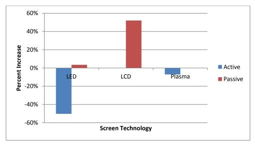
Figure 11: Percent Difference in Luminance from 2D to 3D versus Screen and 3D Technology
