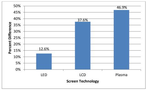
Figure 7: Percent Difference in Power Consumption from 2D to 3D versus Screen Technology
