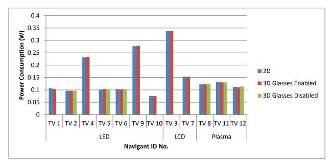
Figure 12: Standby-Passive Power Consumption in 2D, 3D, and 3D with Glasses Disabled
