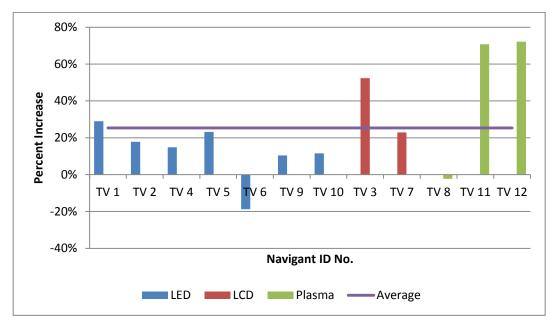
Figure 6: Percent Difference in Power Consumption from 2D to 3D, Separated by Screen Technology
