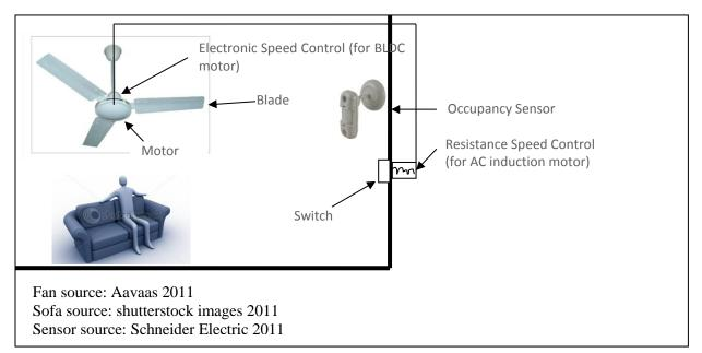
**Figure 1 Ceiling Fan Components**
