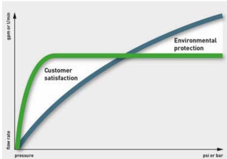
FIGURE 10: PERFORMANCE OF DIFFERENT TYPES OF FITTINGS. THE GREEN LINE SHOWS THE DESIRED PERFORMANCE THAT MAINTAINS A SATISFACTORY FLOW RATE ACROSS A RANGE OF PRESSURES. THE BLUE LINE IS A FITTING TRADITIONAL FIXED-ORIFICE AERATOR WHICH MAY MEET A FLOW-RATE SPECIFICATION AT ONE PRESSURE, BUT DELIVERS UNSATISFACTORY FLOW AT LOWER PRESSURES WHILE WASTING WATER AT HIGHER PRESSURES. 17
