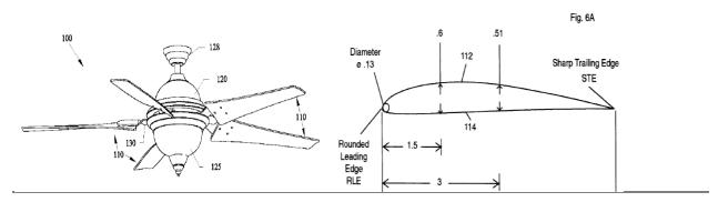
**Figure 1. Design drawings from a patent for a ceiling fan with twisted, tapered blades with an airfoil.** <sup>5</sup> Source: Parker et al. [40]
