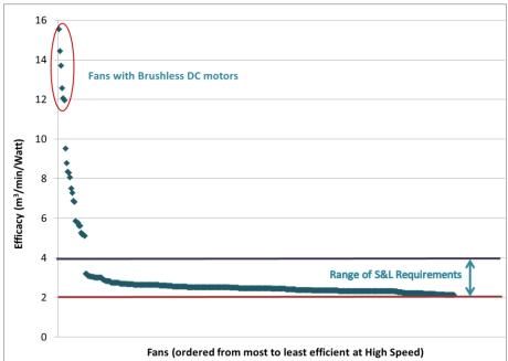
Figure 2. Efficacies for ENERGY STAR ceiling fans (fan only, without lights) at high speed<sup>6</sup>
