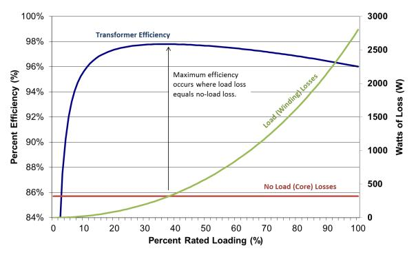
Figure 3-1. Efficiency Changes with Loading, Reaches Peak where NL = LL
