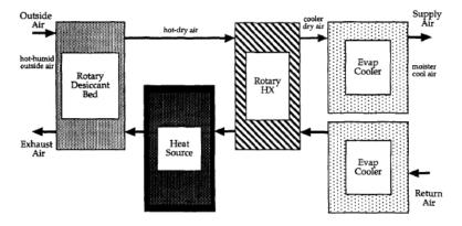
Figure A-3: Air cycle for the desiccant cooling system
