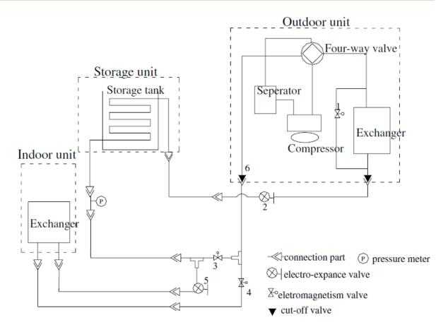
Figure A-8: Schematic diagram of Combined A/C, water heater and energy storage system
