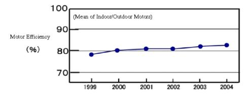
Figure 2-9: Evolution in Japanese air conditioner fan motor efficiency
