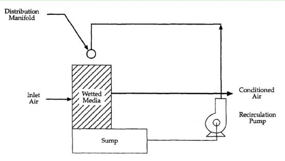
Figure A-1: Typical direct evaporative air conditioner
