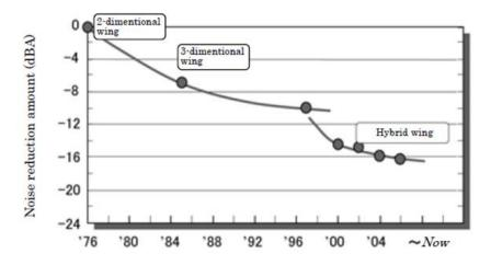
Figure 2-10: Evolution of Axial/Propeller Fan Design
