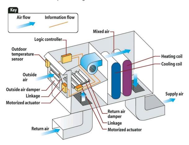
Figure A-7: Diagrammatic Representation of an Economizer
