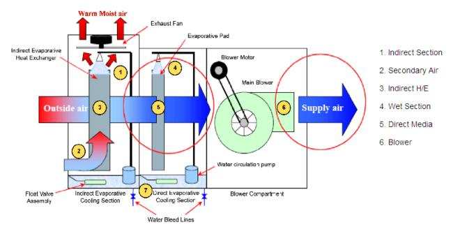
Figure A-2: Indirect-direct evaporative air-conditioning process
