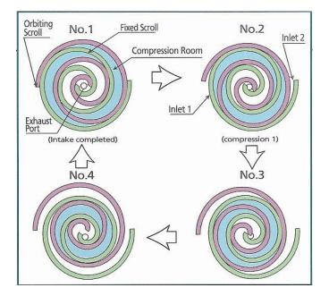
Figure 2-3: Compression cycle in a scroll compressor
