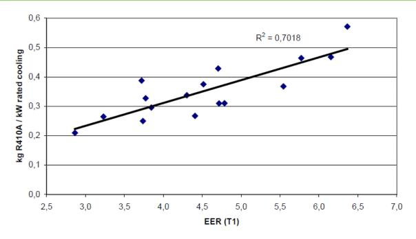
Figure 2-23: Relationship between efficiency and refrigerant charge per kW of cooling capacity
