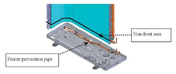
Figure 2-21: Freeze Prevention Pipe for Outdoor Unit Bottom Pipe
