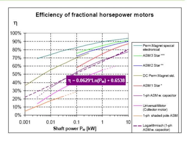
Figure 2-5: Efficiency of fractional horsepower motors
