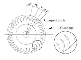
Figure 2-12: Latest Design of Cross Flow Fan Design
