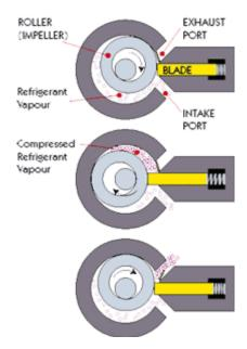
Figure 2-2: Compression cycle in rotary fix-vane compressors
