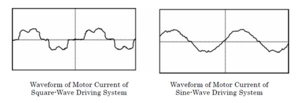
Figure 2-6: Evolution of Motor Current Waveform
