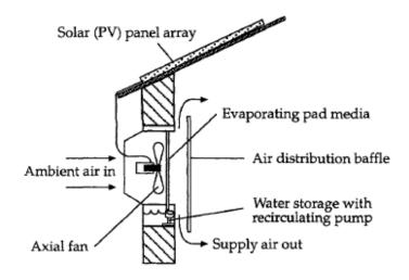
Figure A-5: Solar powered evaporative air conditioner
