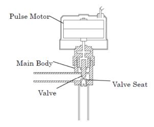
Figure 2-17: Electronic Expansion Valve Schematic
