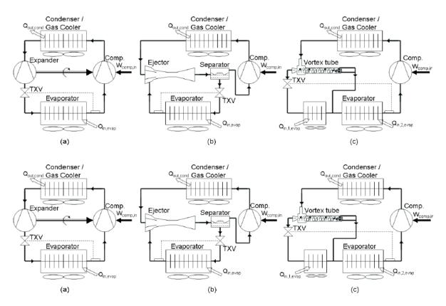
Figure 2-19: Improvement for low ambient heat pump cycle- Expander cycle, (b) Refrigerant ejector cycle, (c) vortex tube cycle
