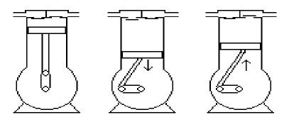
Figure 2-4: Compression cycle in the reciprocating compressor
