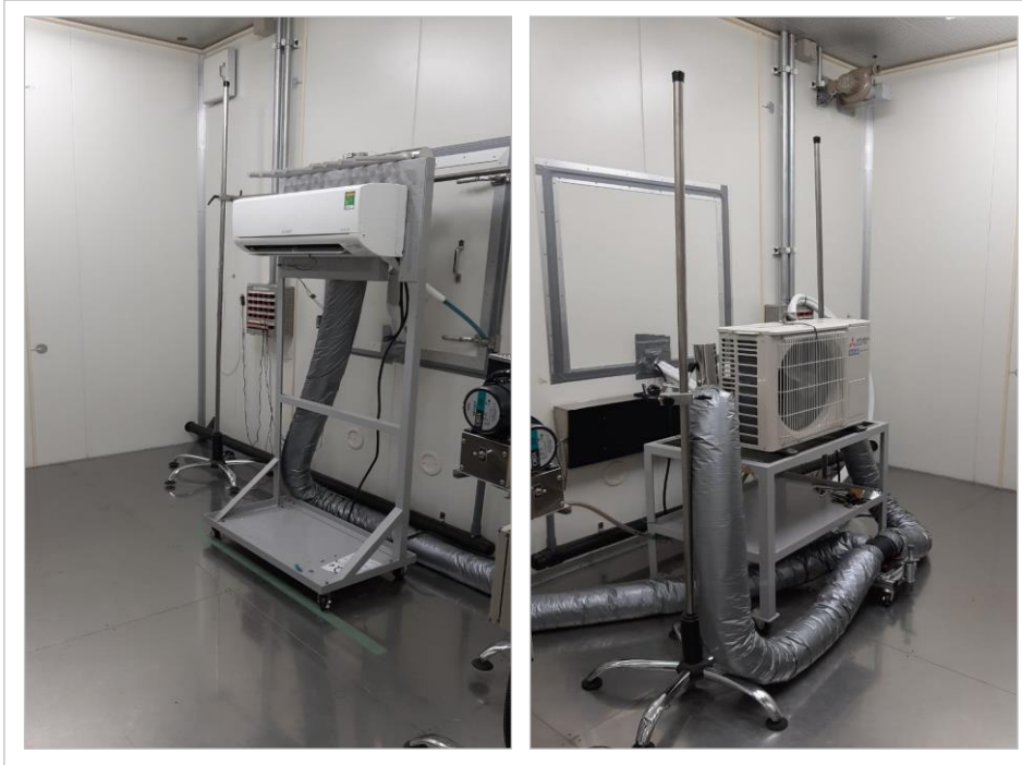
Figure 6. Indoor and outdoor unit set up at one of participating laboratories.
