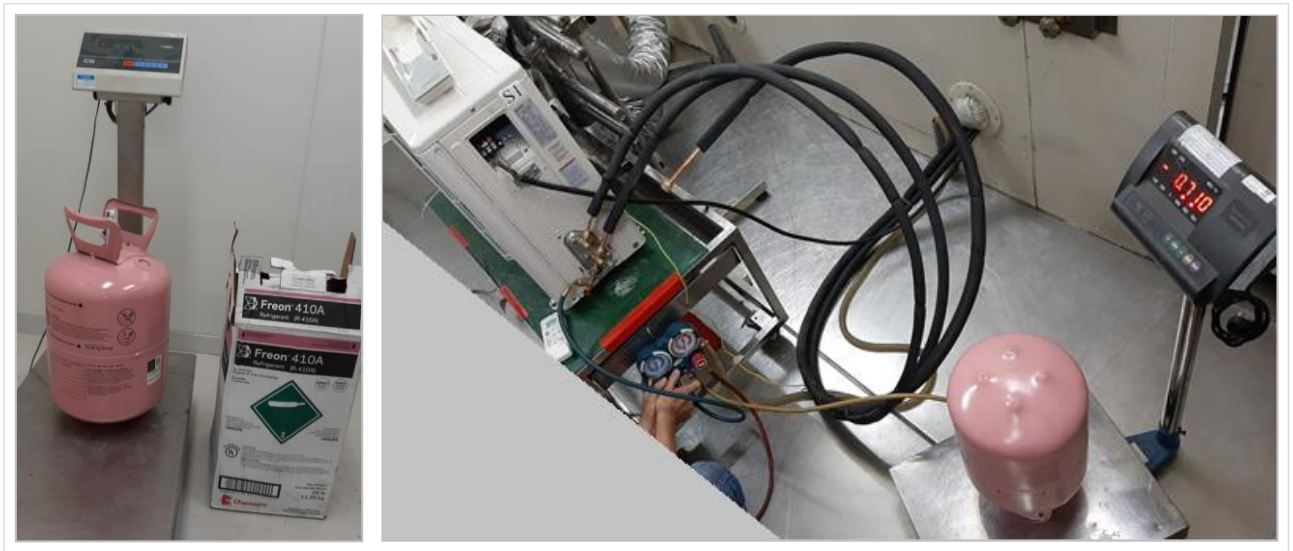
Figure 7. Refrigerant weighting and loading at one of participating laboratories.
