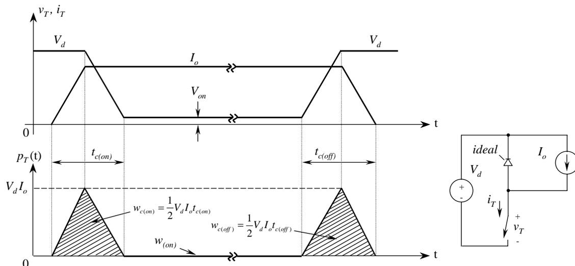
**FigureC-1 — Semiconductor Losses during Commutation Intervals**
