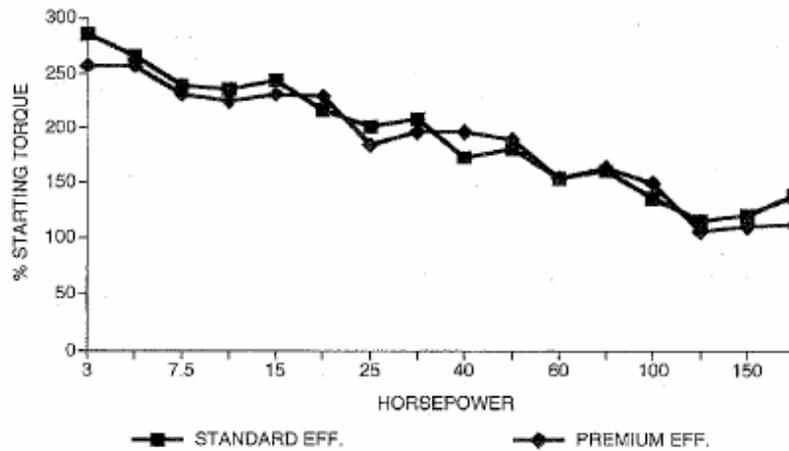
**Figure D-5 - Start-Up Torque of the Motors**
