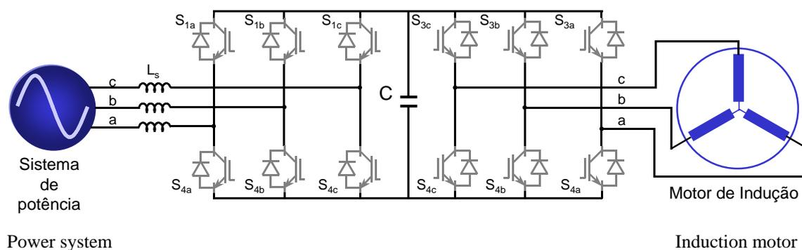
**FigureC-4 — Drive Consisting of Converters with Integrated Gate Bi-Polar Transistor (IGBT) Type Semiconductors**
