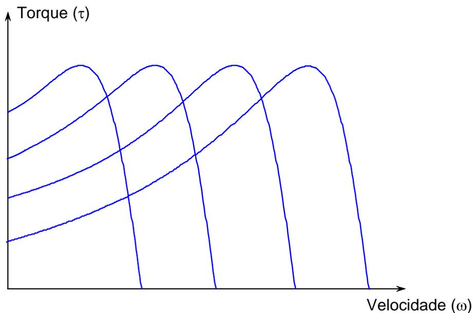
**FigureC-7 — Induction Motor Curves (Torque x rotational speed:  $T \times \omega$ )
