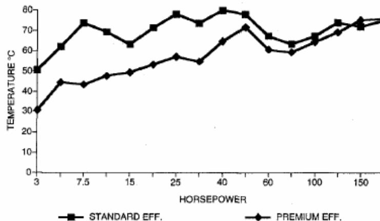
**Figure D-4 - Average Winding Temperatures of Motors in Operation**
