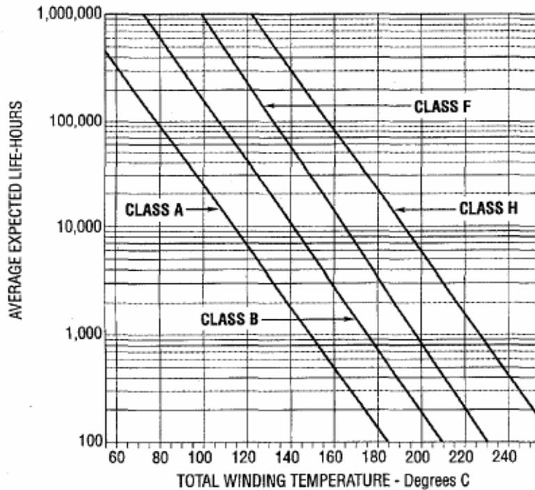
**Figure D-3 - Graph Relating Temperature and Expected Useful Life of Machine in Operation**
