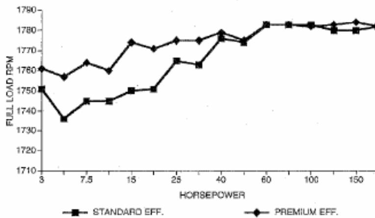
**Figure D-6 - Motor rotation (rpm) at full load.**
