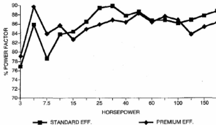
**Figure D-2 - Motor Power Factors**
