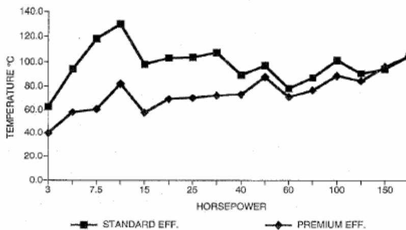
**Figure D-7 - Maximum rotor temperature**
