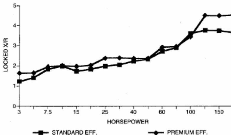
**Figure D-9 - Comparison of the X/R Ratio Between Motors**
