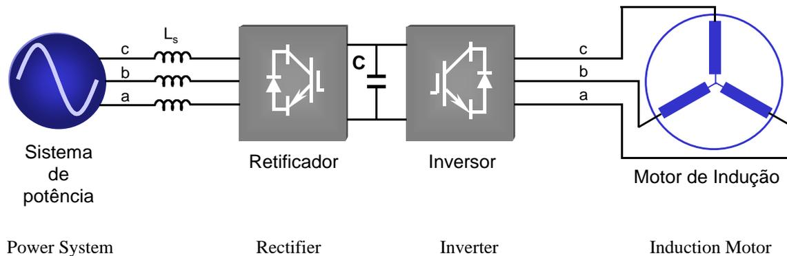
**FigureC-2 — Electronic Drive Consisting of Two Converters Connected Back-To-Back**
