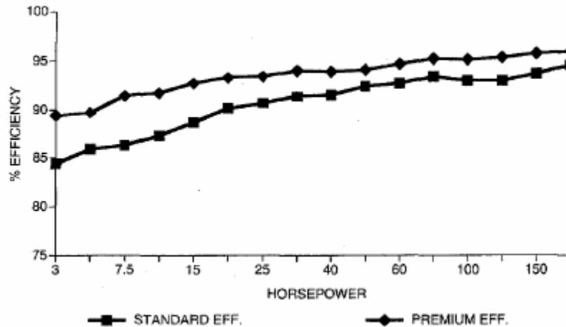
**Figure D-1 - Efficiency of Motors Subject to Similar Conditions**
