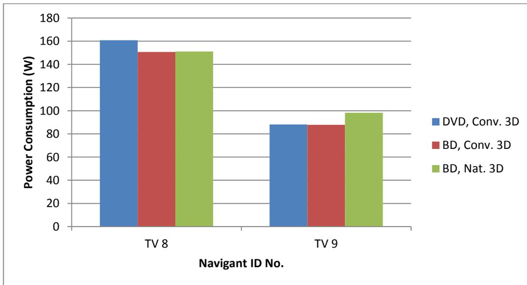
Figure 3: 3D Power Consumption versus Content on TVs 8 and 9
