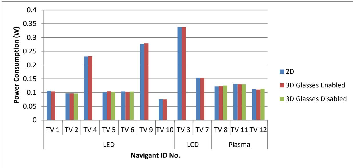
Figure 12: Standby-Passive Power Consumption in 2D, 3D, and 3D with Glasses Disabled
