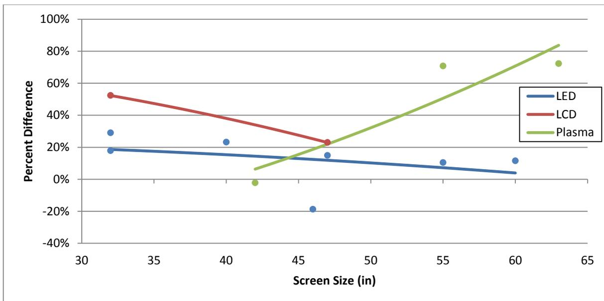
Figure 9: Regression Model - Percent Difference in Power Consumption from 2D to 3D versus Screen Size and Technology
