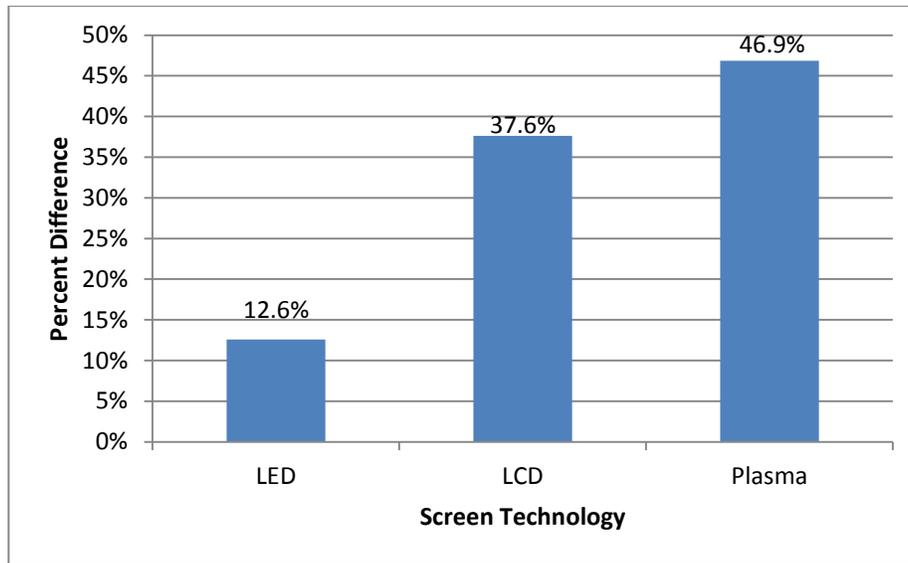
**Figure 7: Percent Difference in Power Consumption from 2D to 3D versus Screen Technology**
