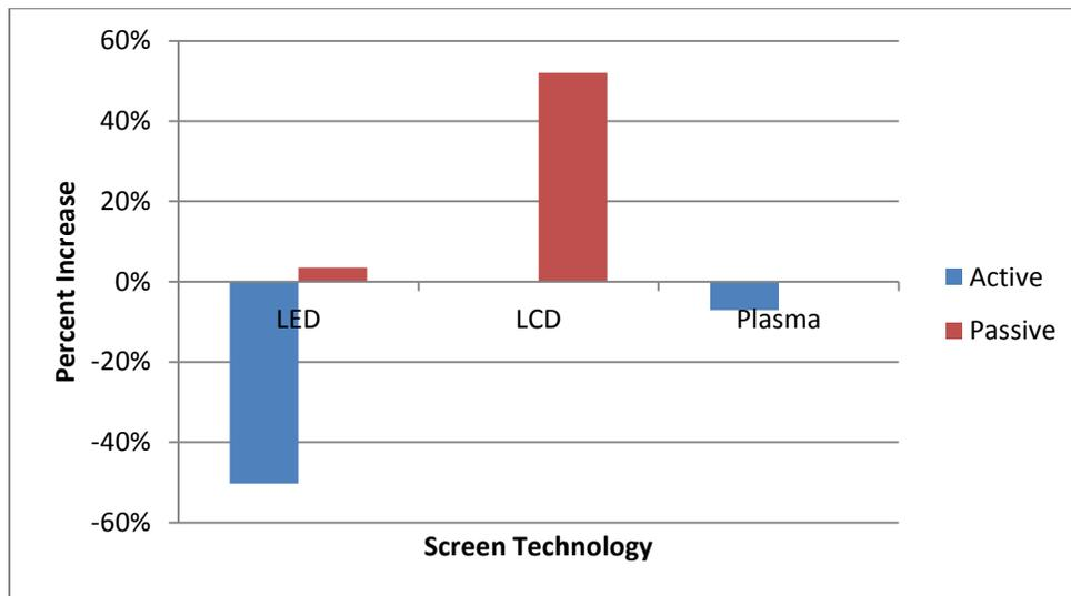
Figure 11: Percent Difference in Luminance from 2D to 3D versus Screen and 3D Technology
