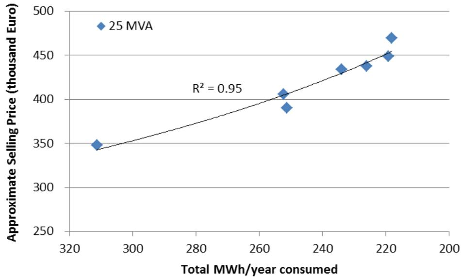
**Figure 1-1. Plot of 25 MVA Transformer, Selling Price versus Energy Consumption**
