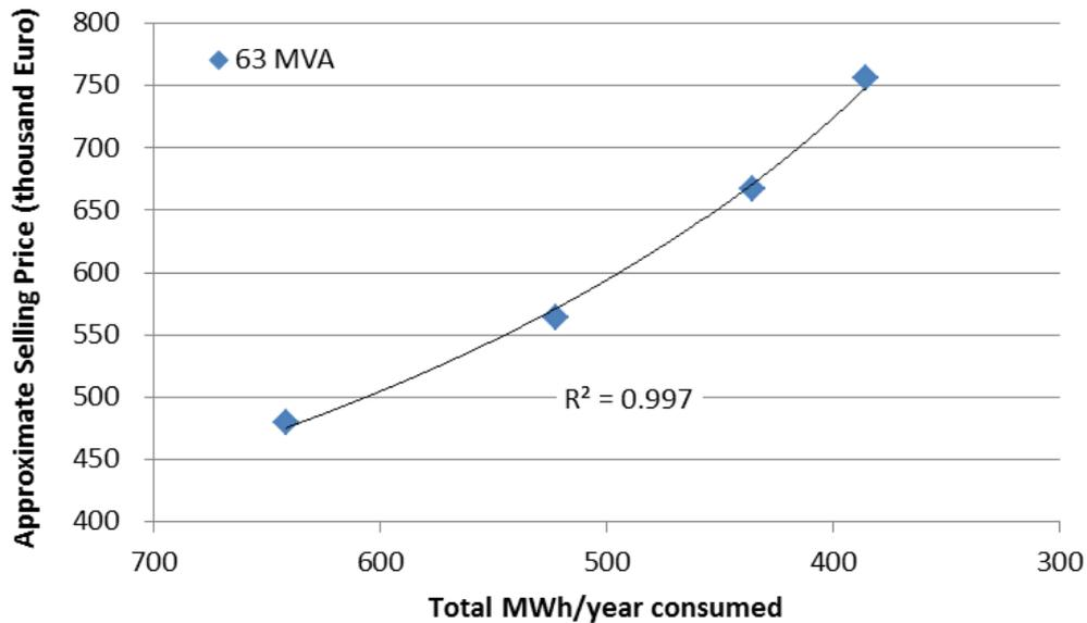
**Figure 1-2. Plot of 63 MVA Transformer, Selling Price versus Energy Consumption**
