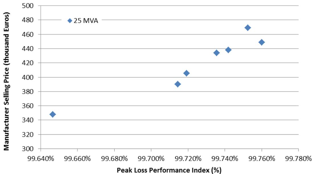
**Figure 2-1. Selling Price vs. Peak Loss Performance Index for 25 MVA Transformer**
