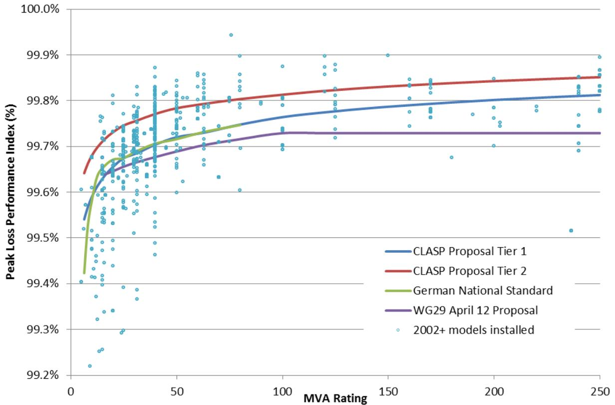
**Figure 1-8. CLASP Proposed Regulatory Requirements for Large Power Transformers and Comparison to 2002-2012 Market**
