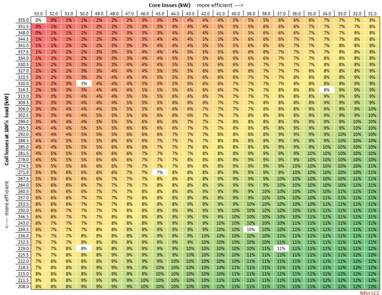
Figure 1-7. Life-Cycle Cost Savings Matrix for the 100 MVA Transformer
