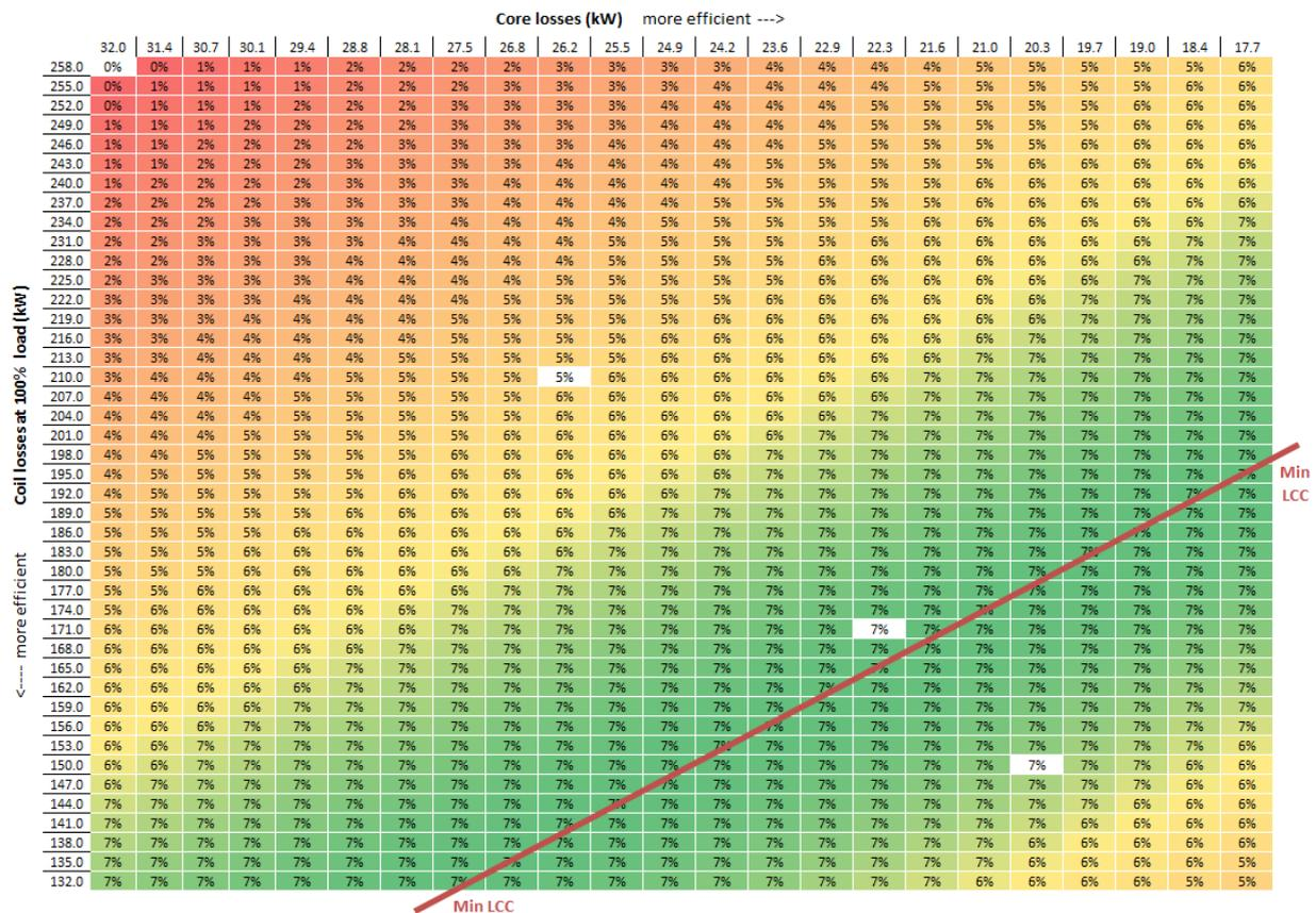
Figure 1-6. Life-Cycle Cost Savings Matrix for the 63 MVA Transformer
