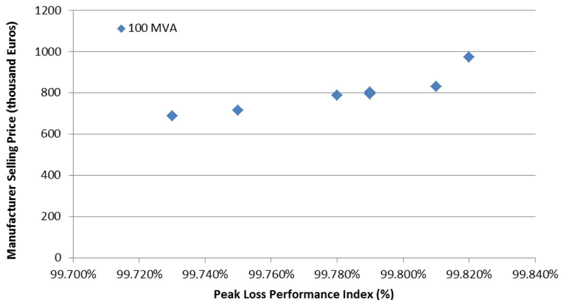
**Figure 2-3. Selling Price vs. Peak Loss Performance Index for 100 MVA Transformer**
