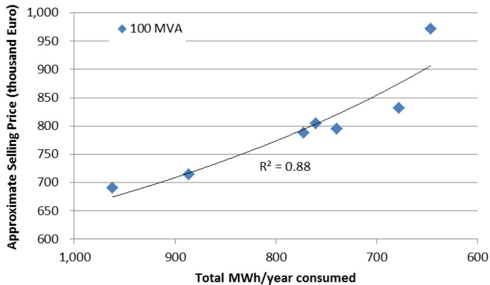
**Figure 1-3. Plot of 100 MVA Transformer, Selling Price versus Energy Consumption**
