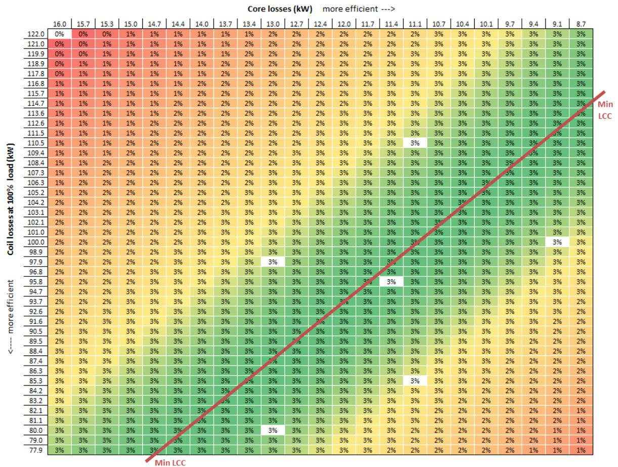
**Figure 1-5. Life-Cycle Cost Savings Matrix for the 25 MVA Transformer**
