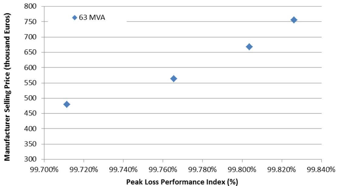
**Figure 2-2. Selling Price vs. Peak Loss Performance Index for 63 MVA Transformer**
