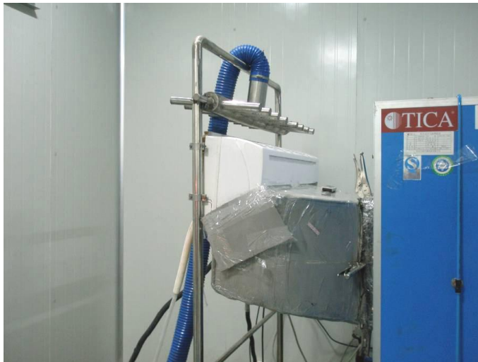
Figure 9 Air Enthalpy Method at Laboratory 3
