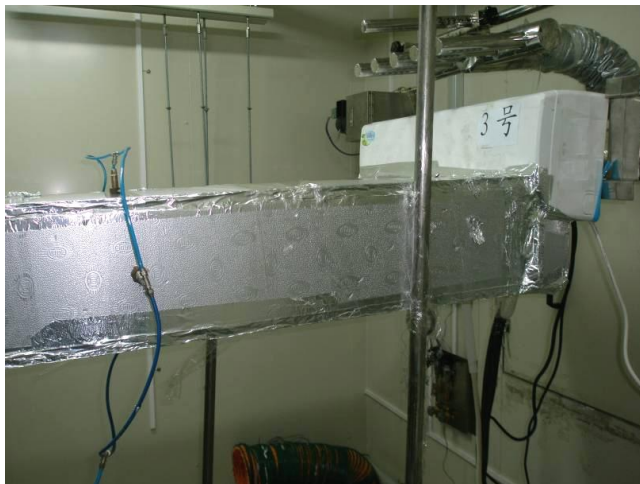
Figure 8 Air Enthalpy Method at Laboratory 2
