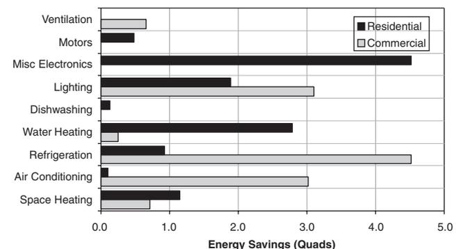
Fig. 3. Cumulative primary energy savings from upgraded standards for products installed in 2010–2030 period.
