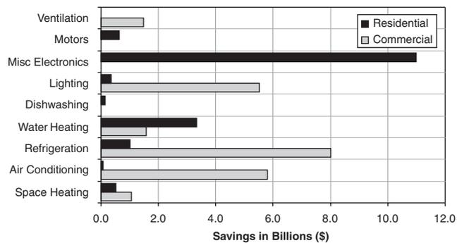
Fig. 4. Net present value of consumer benefit from upgraded standards for products installed in 2010–2030 period (7% discount rate).
